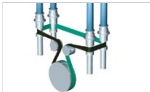
W-8/DS-8 four-spindle drive with two jockey pulleys
